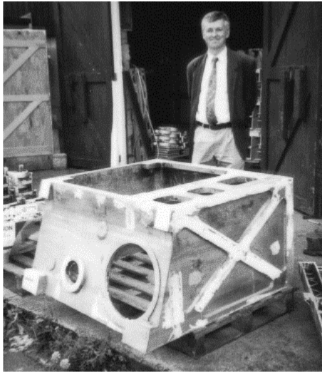
Figure 10. Michelle Vacuum Vessel - Centre Section Casting. Size approx 1.2m square by 0.75m deep.
