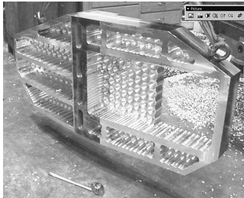
Figure 1: Altair optical bench after rough machining.
