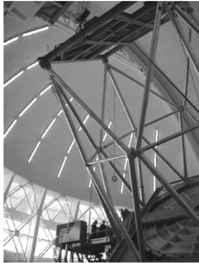
Figure 4: Cerro Pachón telescope being tilted. Note the dummy mirror being held in the telescope with the mirror cell and support system.
