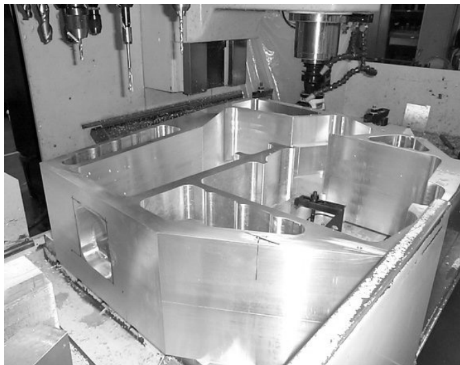
The main optical bench of GNIRS undergoing machining at NOAO during the week of March 20, 2001.
