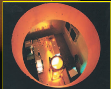
A view down the custom cut exit hole for the dye laser used in this experiment. The laser is located in a utility building below the Blanco Telescope on Cerro Tololo
