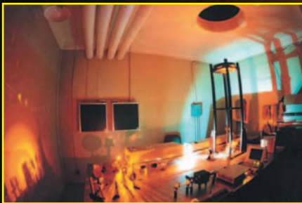
An inside view of the laser room showing the 0.4 mW dye laser and 7W Argon-ion pump laser that is tuned to the Na D2 line for this experiment. The exit hole can be seen on the room's ceiling.
