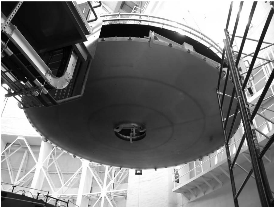
Figure 4: Gemini South Primary mirror being lifted after receiving its first coating.
