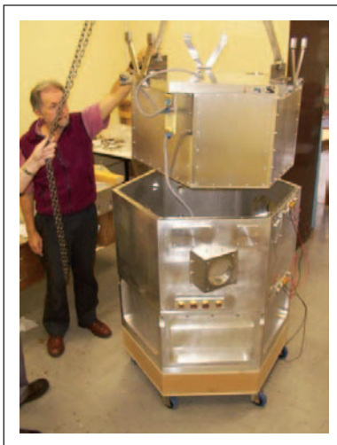
Peter Conroy lowering the cold work surface plate into the cryostat.
