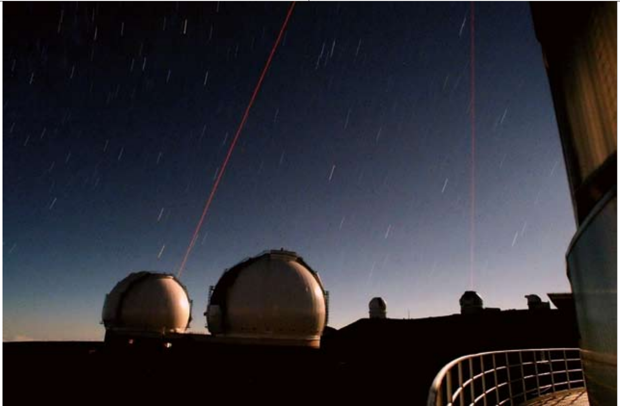
Gemini and Keck laser guide star propagation captured by Akihiko Miyashita from the Subaru Observatory
