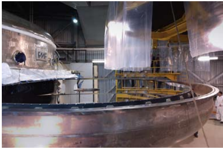
Figure 1. The Gemini South mirror as it emerges from the coating chamber with a fresh coat of protected silver. The coating technology developed at Gemini has resulted in highly durable coatings that have exceeded expectations in performance and is being adopted by other projects like the Thirty Meter Telescope currently under development.
