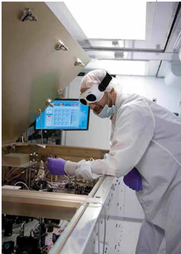
Figure 4. Gemini laser specialist Vincent Fesquet, wearing laser safety goggles and clean room clothes, aligning the Gemini South laser bench in the Laser Service Enclosure. Gemini photo by M. Paredes.
