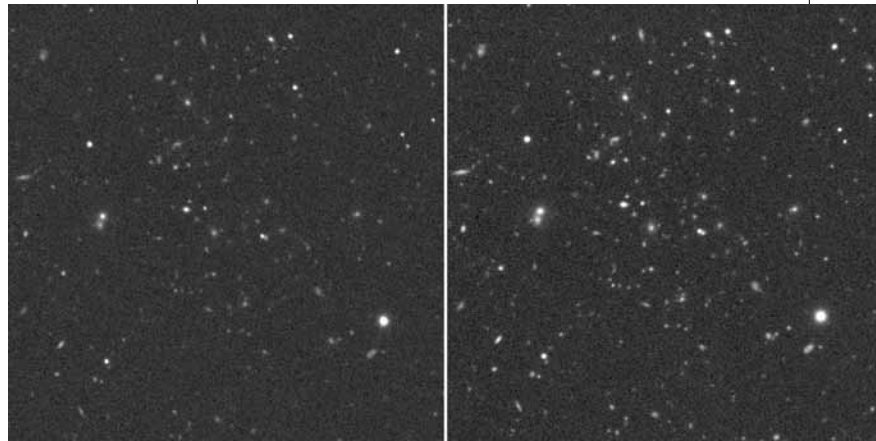
Figure 3 (center). An old GMOS-North CCD image on the left (60-minute exposure, seeing = 0.55 arcsecond full-width at half-maximum (fwhm)), and a new GMOS-North CCD image on the right (55-minute exposure, seeing = 0.54 arcsecond fwhm). Both images use the same z-band longpass filter and the stretch is identical. In the z-band, the gain in sensitivity is ~ 0.5 magnitude (about a factor of 3) according to preliminary analysis of data. The z-band is broad and red, so it shows the greatest improvement in sensitivity; other filters will show smaller gains.
