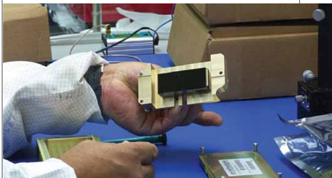
Figure 4 (bottom). One of three new GMOS-North CCD E2V Deep Depletion CCDs with increased red sensitivity.
