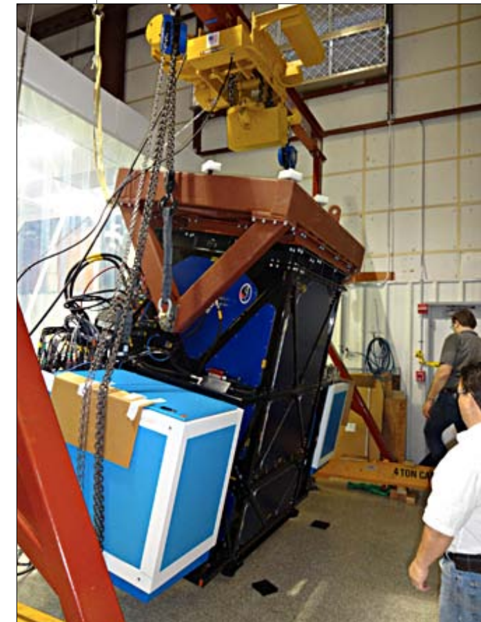
Figure 5. The Gemini Planet Imager being tested on the flexure rig at the University of California Santa Cruz.
