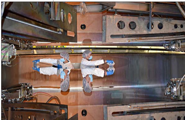
Figure 1. The Gemini North 8-meter primary mirror is inspected inside of the coating chamber.
