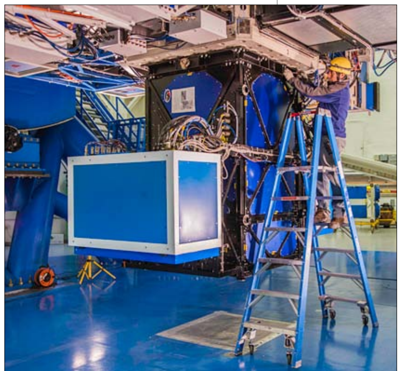
Figure 2. GPI is mounted on the Gemini South telescope prior to first light observations in late 2013.
