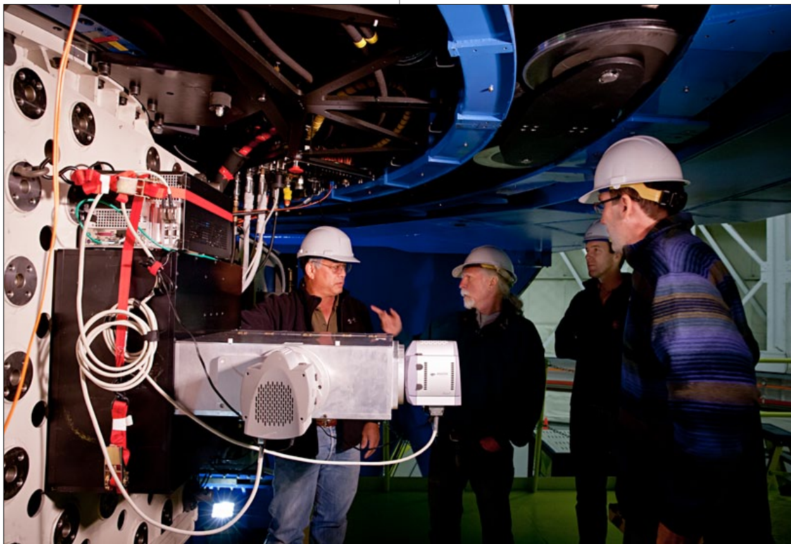
Figure 3. The Gemini North visiting instrument DSSI (Differential Speckle Survey Instrument) being mounted on the Instrument Support Structure of the Gemini North telescope during an observing run in 2103.
