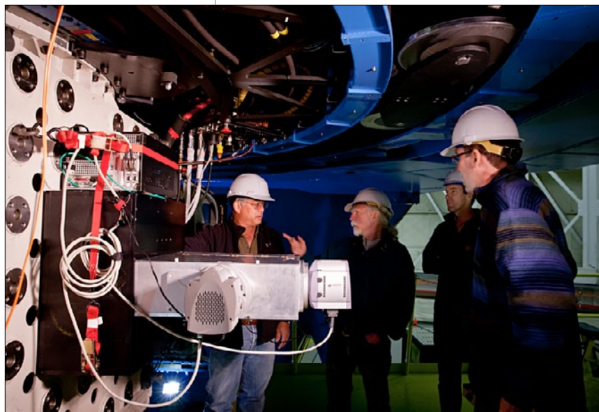
Figure 14. The Gemini North visiting instrument DSSI (Differential Speckle Survey Instrument) being mounted on the Instrument Support Structure of the Gemini North telescope during an observing run in 2013.
