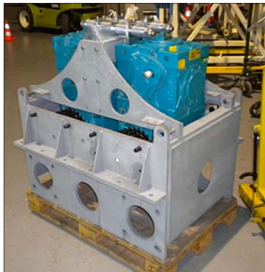
Figure 1. A fully assembled, spare shutter gearbox at Gemini North. Redesigned torque arms are at the top of the assembly.
