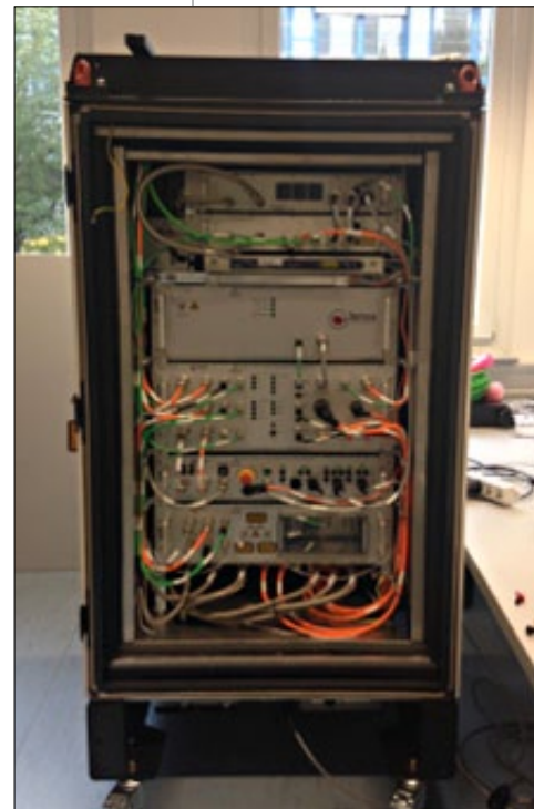
Figure 5. The Gemini South laser cabinet just before connecting to the laser head during the FAT readiness review on October 5-6. Image credit: All three images by Manuel Lazo
