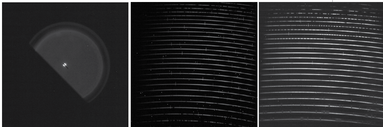
Figure 1. IGRINS+Gemini South first light. Left: TW Hydrae in the slit-viewing camera. Center: the H-band spectrum. Right: the K-band spectrum. Credit: K. Sokal and the IGRINS team
