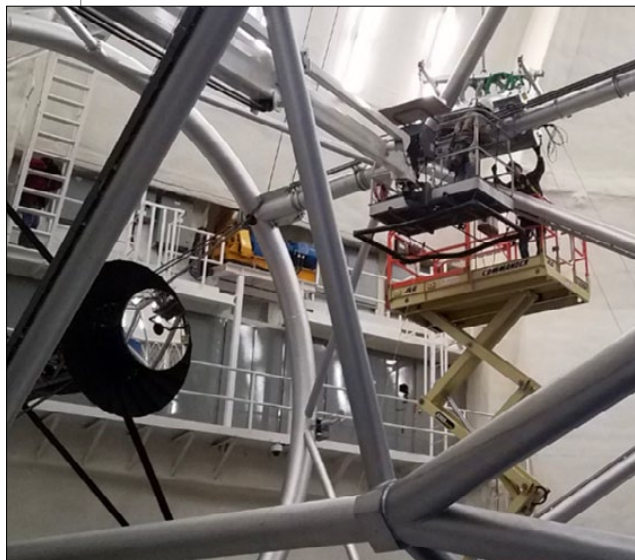
Figure 8 (above right). Verifying laser alignment through the optical path to the Beam Transfer Optics Optical Bench on the secondary.
