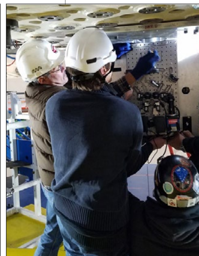
Figure 3 (left). Harlan Uehara (left) and Gemini North’s Senior Instrumentation Engineer John White (right) position the ballast weight assembly so that it attaches to the instrument port around HIPPI-2. The ballast weight is necessary to balance the telescope because HIPPI-2 weighs much, much less than the facility instruments!
