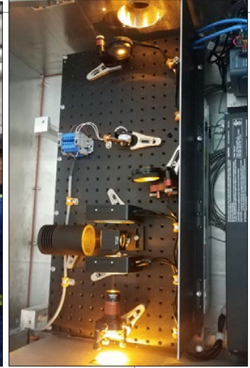
Figure 7 (above left). Gemini Optical Engineer Tom Schneider prepares insulation for GNEST (laser housing designed for our TOPTICA laser head and optical bench).
