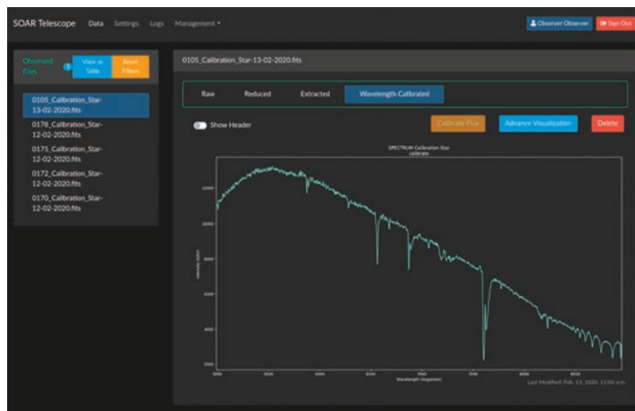
Figure 4: Screenshot of the web-based interface to the Python live Goodman spectroscopic pipeline, showing a fully reduced spectrum of a standard star. It features basic interactive visualization tools that allow zooming into particular regions, coordinates of the mouse position, and saving a view to a png file. Analysis capabilities such as equivalent width and signal-to-noise measurements will be added in future versions.
