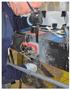
Figure 3: Removal of the Pad L10 from GN M1 by Jean-Benoît de Vanssay. Credit: Safran-Reosc
