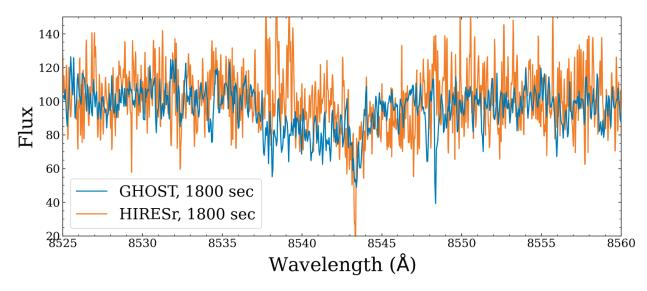
Figure 2: An example spectral comparison for the White Dwarf WD 1145+017 from GHOST and the High Resolution Echelle Spectrometer (the long-wavelength configuration; HIRESr) on Keck I. WD 1145+017 is the first white dwarf discovered to show transits from a disintegrating asteroid [2]. Its atmosphere is heavily polluted from accretion of the circumstellar material and GHOST SV data will be used to constrain the evolution of that material over time. *Credit: NOIRLab/AURA/NSF/S. Xu*
