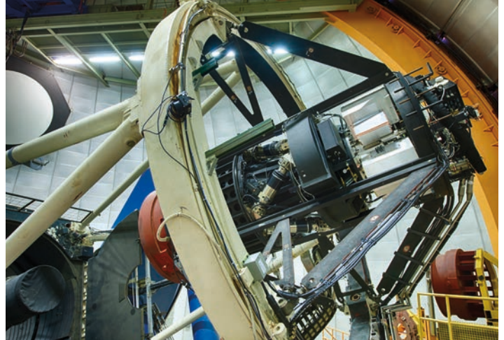
Figure 2. DECam on the Víctor M. Blanco 4-meter Telescope. Credit: Reidar Hahn, Fermilab
