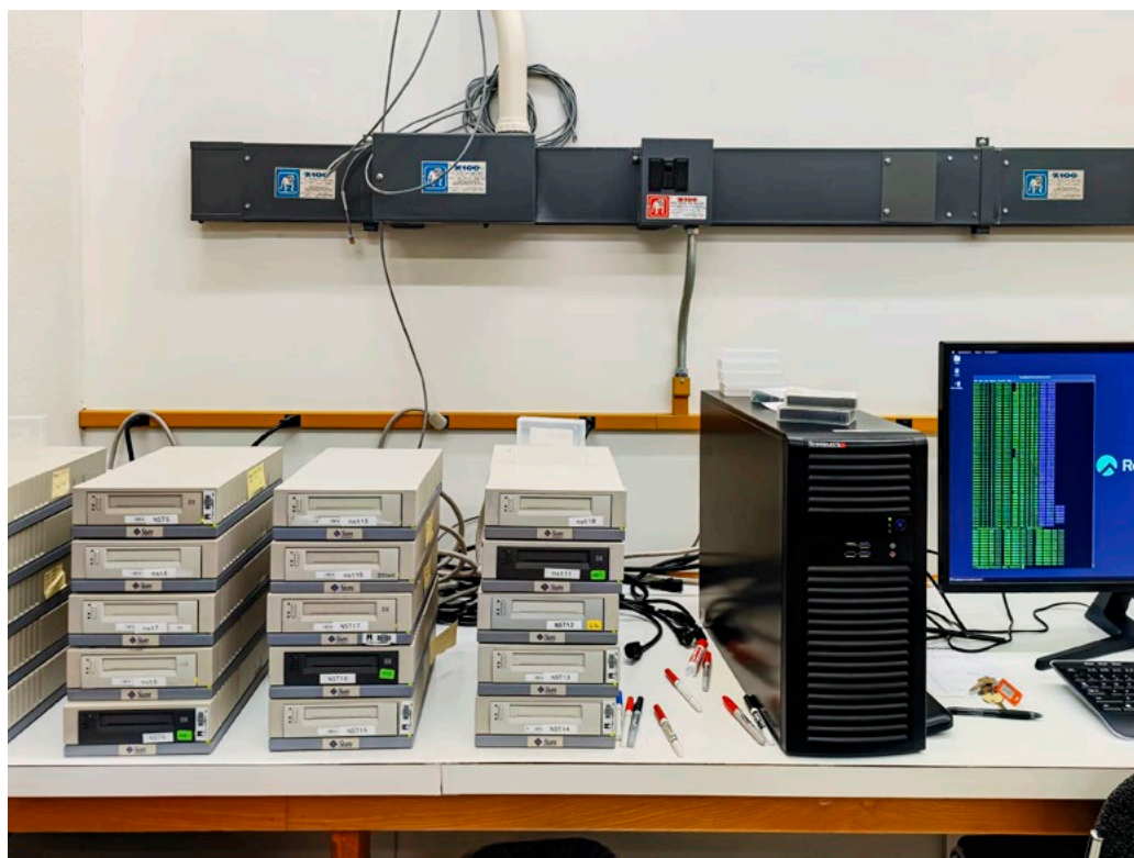
Figure 1: Exabyte tape drives for the Astro Data Legacy Tape Drive Archive. Credit: R. Faux/NOIRLab
