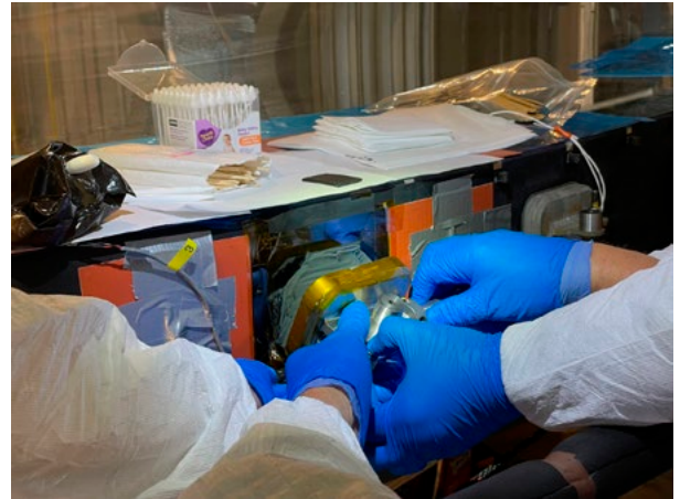
Figure 6: NOIRLab M1 repair team members placing the new L10 lateral pad into position on the Gemini North primary mirror. Credit: NOIRLab/NSF/AURA/Katie Smither
