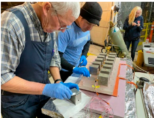
Figure 5: NOIRLab GN M1 team members Gary Pozculp, Tom Schneider, and Heather Carr prepare witness samples to test the L10 epoxy application and bonding to ULE glass block. Credit: NOIRLab/NSF/AURA/Katie Smither
