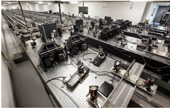
Figure 4: Beam synthesis facility. Optical delay room. The variable delay lines extend toward the upper left. Metrology, beam compression, switching, and dispersion compensation are on the tables in the foreground. Credit: S. Golden/Georgia State University
