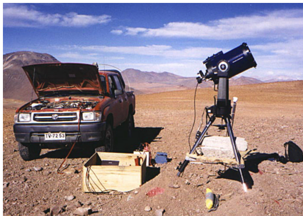
Atmospheric seeing measurements are being made in the Atacama desert of Chile to characterize sites for the Giant Segmented-Mirror Telescope. A robotically controlled differential image motion monitor (DIMM) was used on the 5400-m (17,500 ft) summit of Cerros de Honar. (Photo: Brooke Gregory)
