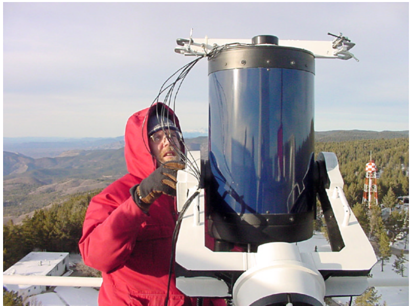
Site Survey Working Group Chair Frank Hill with the ATST S-DIMM/scintillometer array mounted on top of the Dunn Solar Tower at Sacramento Peak. The two large holes (left panel view of the instrument) are the entrance apertures for the S-DIMM; the bar across the center holds the six scintillometers.
