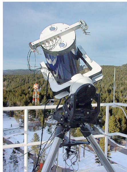
Site Survey Working Group Chair Frank Hill with the ATST S-DIMM/scintillometer array mounted on top of the Dunn Solar Tower at Sacramento Peak. The two large holes (left panel view of the instrument) are the entrance apertures for the S-DIMM; the bar across the center holds the six scintillometers.
