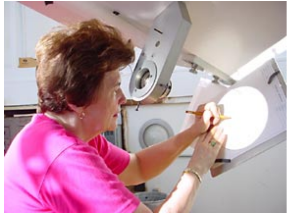
Mary Bishop, a high school science teacher from New York, carefully sketches all sunspots visible on a projected solar image during the July 2002 TLRBSE workshop. Such sketches are done each sunny day in the Hilltop Dome at Sacramento Peak Observatory as part of the dawn "Flare Patrol." Mary and her fellow teachers made solar sketches using the patrol telescope as part of their research experience in Sunspot, NM.
