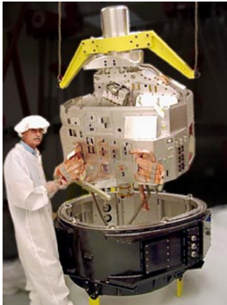
Figure 1. The GNIRS optical bench is lowered into the dewar shell as a fit check, with guidance from GNIRS Project Support Scientist Dick Joyce.
