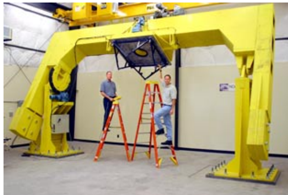
Figure 2. The newly installed NOAO Flexure Test Facility will be used to test GNIRS for flexure. GNIRS mechanical engineers Ed Hileman (left) and Gary Muller are shown fit testing the GNIRS ISS interface assembly.
