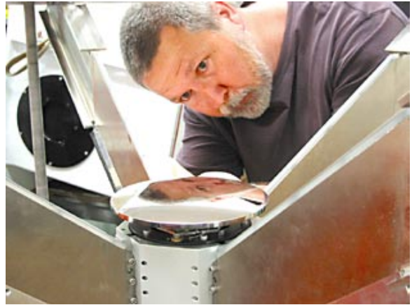
Gary Poczulp installs the secondary mirror of the SOLIS Vector Spectromagnetograph Ritchey-Chretien telescope. The mirror is mounted on a piezoelectric tip-tilt mechanism that allows correction of image motion up to \pm 55 arcsec. The spider that holds the mechanism is inverted here.
