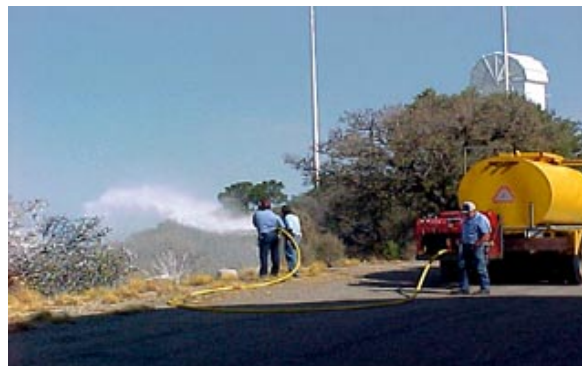
KPNO facilities crew tests foaming pump for fire protection.
