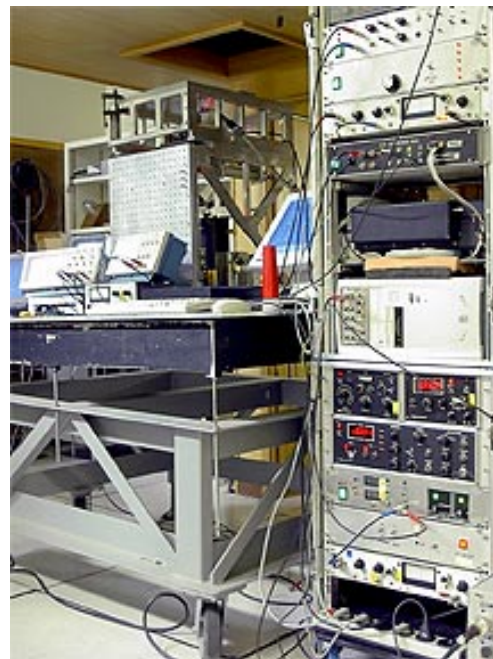
Figure 1: THIS at the McMath-Pierce West Auxiliary Telescope. The cubic aluminium structure on the left is the optical receiver; the 19-inch rack on the right holds the AOS and back-end electronics.
