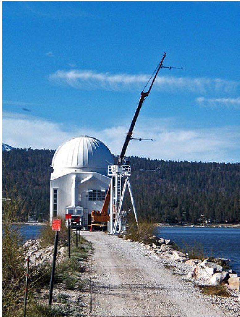
Figure 2. Comparison test of in situ and ATST measurements of seeing as a function of height underway at Big Bear.
