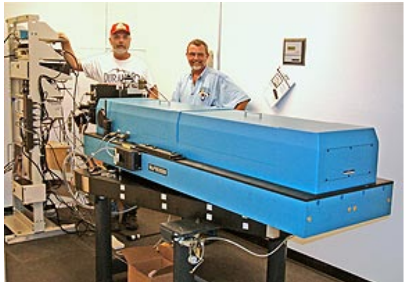
The two-meter focal length, double-pass Integrated Sunlight Spectrometer (ISS) is now installed in a temperature-stabilized room in the Kitt Peak SOLIS Tower (KPST). The rack at the left contains control electronics and lamps that feed light into the instrument via optical fibers. Shown here with the ISS are (from left) Ed Stover (NSO/SOLIS) and Mike Hawes (NOAO).
