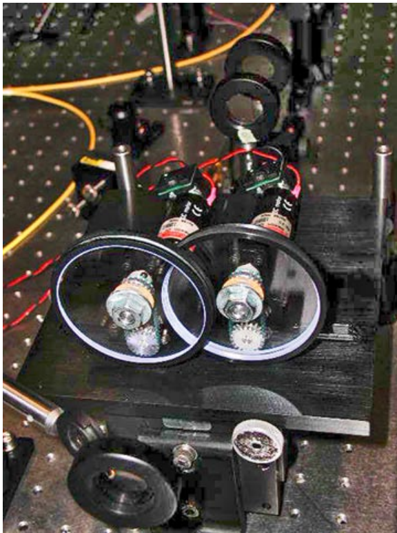
Figure 2: The prototype simulator installed in the laboratory, with the disks mounted on a rigid platform, as they will be mounted in the TurSim module for SAM. Each disk is connected to its own DC motor, with variable speed.
