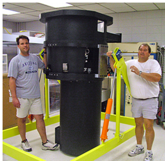
FLAMINGOS-2, supported vertically in its handling and flexure-testing cart, is shown with University of Florida engineering team members Jeff Julian (left) and Greg Bennett (right).
