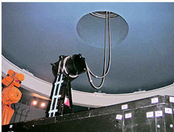
The bHROS fiber bundles emerge from the bottom of the pier of the Gemini South telescope and enter the climate-controlled bHROS enclosure.
