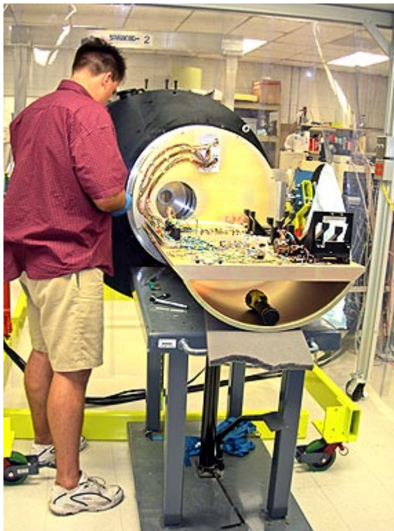
The FLAMINGOS-2 camera dewar optical bench, with Florida engineer Jeff Julian working. The dewar wiring is visible.
