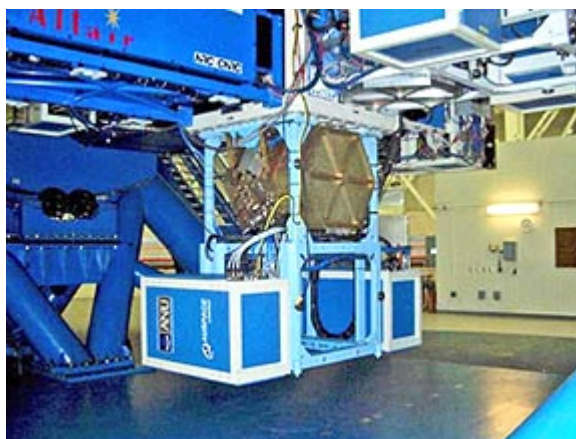
Figure 1. NIFS mounted on the up-looking port of the Gemini North telescope. The hexagonal cryostat is a copy of the NIRI design. The electronics for instrument control, the detector, and the on-instrument wavefront sensor are deployed in the two blue environmental cabinets mounted with the cryostat. The Altair facility adaptive optics system is mounted on a side port above NIFS (Photo credit: Peter McGregor and Gemini).
