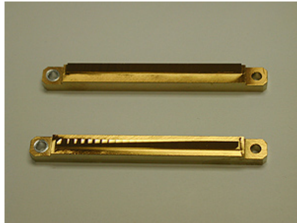
Figure 1. The slit-mirror array (top) and pupil-mirror array (bottom). Each array consists of 25 individual mirrors that are made on a monolithic aluminum-alloy substrate.
