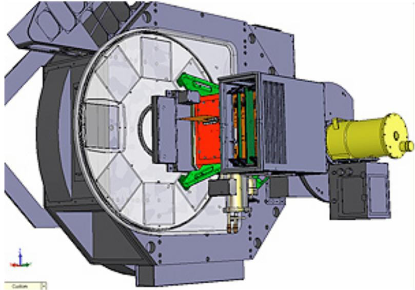
Figure 1. Rendering of QUOTA at WIYN's imaging port, with WTTM to the right.
