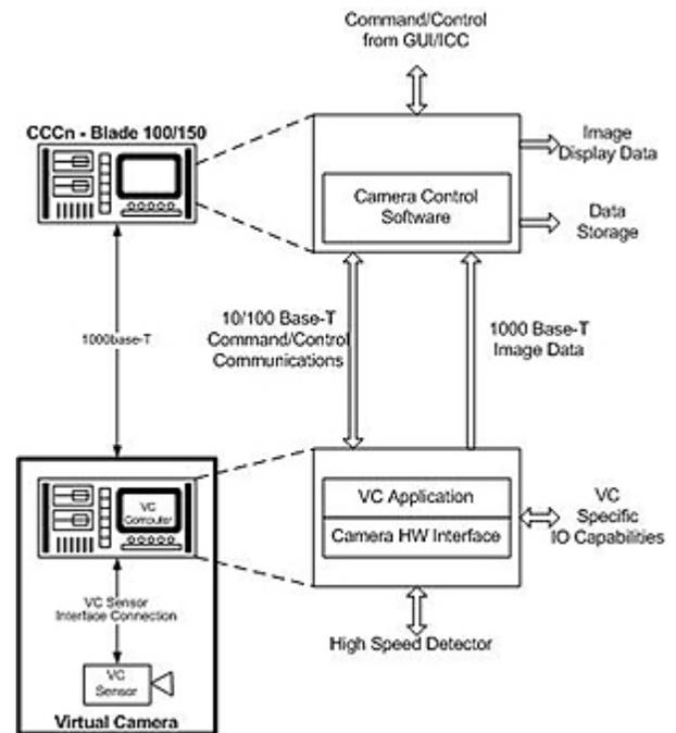
*Schematic of the NSO Virtual Camera System at the Dunn Solar Telescope.*
