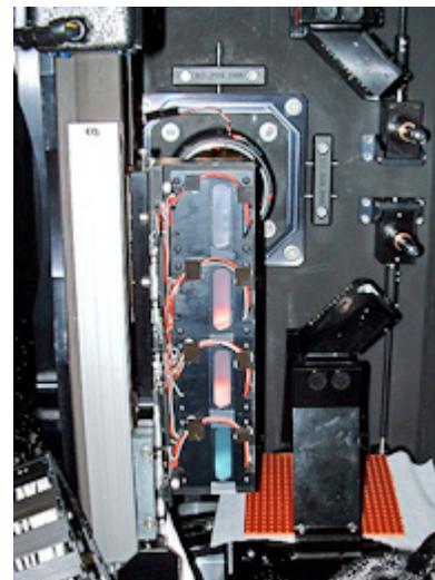
Figure 2. View of the modulator assembly inside the VSM from the back end looking toward the corrector optics (black housing in front of modulator assembly). The translation stage for the assembly is on the left, and the perforated sheet (lower right) protects the Offner mirror.
