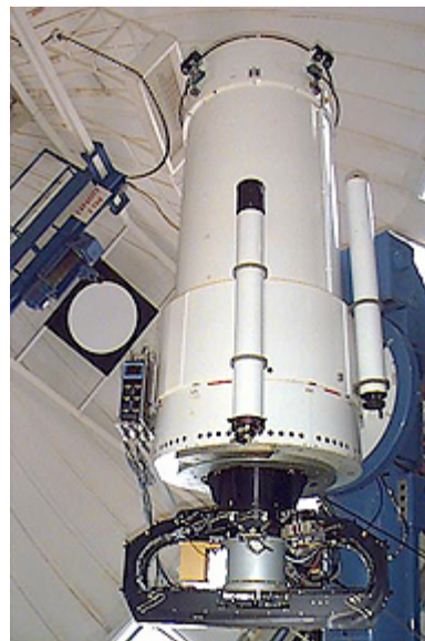
The KPNO Mosaic camera is available for use with the WIYN 0.9-meter telescope (above), but is primarily used with the Mayall 4-meter telescope. With the 0.9-meter, Mosaic provides a one-degree field of view with approximately 0.6-arcsecond pixels. The new Half-Degree Imager, while providing only a 0.5-degree field of view, will have smaller pixels (0.43 arcseconds), a better match to the good image quality provided by the telescope and the site.
