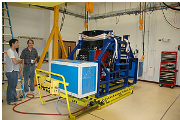
Figure 2. Gemini Observatory Director Doug Simons (right) inspects the new NICI instrument on a Gemini standard instrument air pallet in the Gemini Hilo Base Facility instrument bay, where it will undergo flexure testing.
