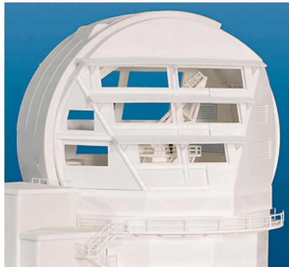
Figure 1. The model of ATST, produced on a 3-D printer by Solid Concepts, illustrates the ‘exoskeleton’ configuration for the carousel structure, skin, and plate coil.
