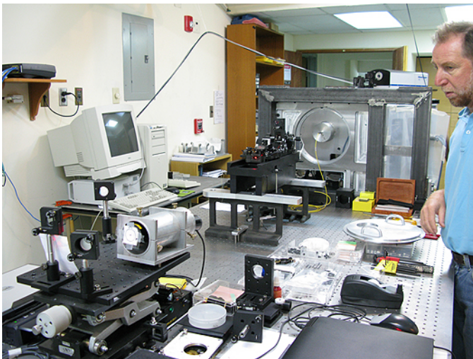
TurSim mounted into the SAM Main Module (left), and Optical Engineer Roberto Tighe working on the integration and alignment of TurSim.
