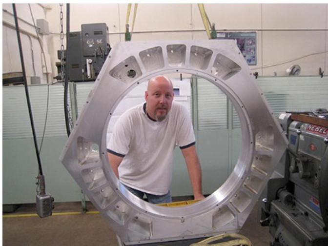
Figure 1: Instrument maker, Ron Harris, standing behind the aluminum Atmospheric Dispersion Compensator (ADC) housing. Three triangular shaped outrigger blocks will bolt to the housing to form the main structural component to which filter mechanisms and axles, ADC cells, and Dewar will mount. When completed, the housing will weigh 170 pounds with overall dimensions of 37 inches across the flats by 6.26 inches thick.
