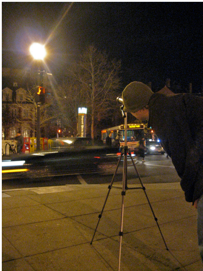
Figure 1: Galileoscope being used for viewing Venus (through the tree) for an urban star party at Dupont Circle in Washington DC. The telescope was designed for good stray light rejection to encourage its use in large cities. (Photo S. Pompea)
