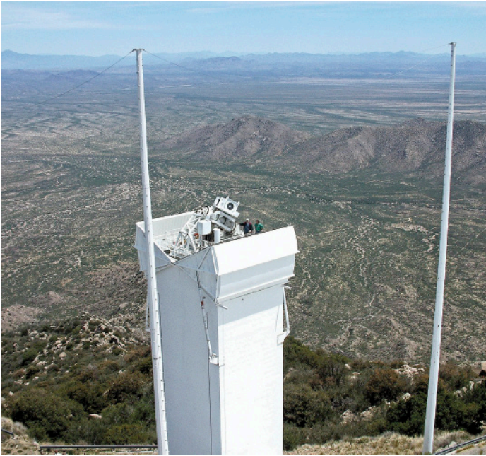
Figure 3: SOLIS mount and the Vector Spectromagnetograph (VSM) instrument installed at the Kitt Peak SOLIS Tower (formerly the Vacuum Telescope) surrounded by lightning protection towers. (Image credit: Kevin Schramm/NSO/NOAO/NSF.)
