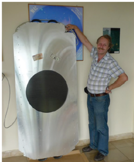
Figure 1: The DECam shutter. At 600 mm clear diameter this is the largest “Bonn shutter” ( www.astro.uni-bonn.de/~ccd/shutters/ ) yet made. (Image credit: Argelander-Institut für Astronomie.)
