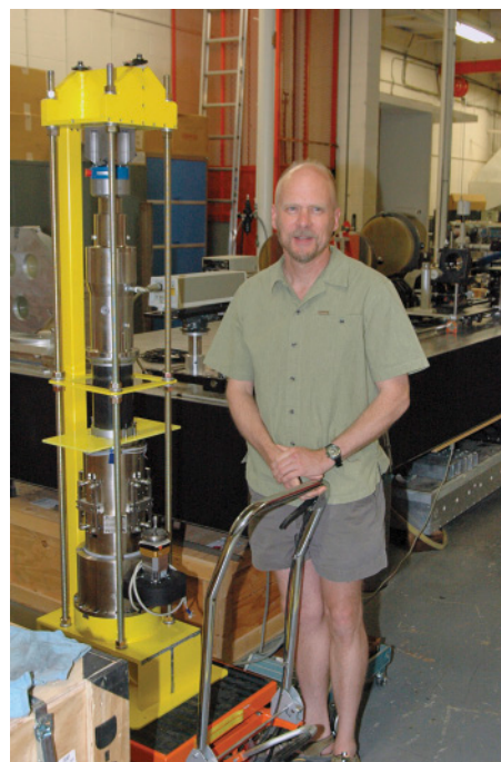
Figure 4: Joe DeVries with the LSST primary mirror hardpoint strut.
