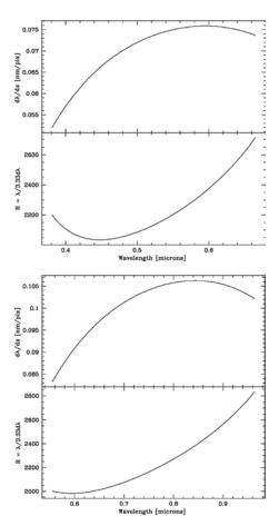
Figure 1: Dispersion curves for the blue (top) and red (bottom) grisms. The resolution shown is specified for a 1-arcsec slit, but the slits that will be provided will actually be 0.6, 0.9, 1.2, and 1.8 arcsec wide, plus a wider slit for photometric calibrations. The instrument image quality should allow use of the 0.6-arcsec slit for those willing to accept the associated light losses at the slit.
