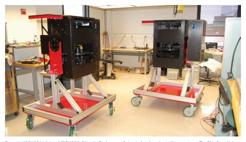
Figure 2: KOSMOS (right) and COSMOS (left) in the final stages of electrical and mechanical integration at The Ohio State University in Columbus, Ohio. The spectrographs are shown on their handling carts in the up-looking position, which is the same way they will mount in the cass cages of the 4-m telescopes using an adapter that is not shown. The Dewars install on the bottom of the instruments. Various covers are not yet installed in these photos.
