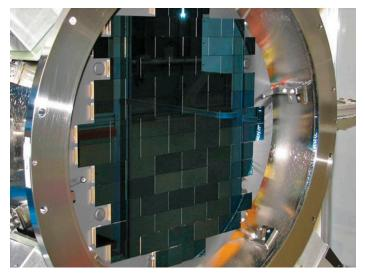
Figure 1: The Dark Energy Camera (DECam) focal plane with all 74 science-grade CCDs installed. On the Blanco Telescope, the 45 cm diameter focal plane covers 3 square degrees of sky, (12 times the area of the Full Moon). The fully depleted back-illuminated CCDs were made at LBL and packaged, tested, and installed at Fermilab. (Image credit: Juan Estrada, Fermilab).
