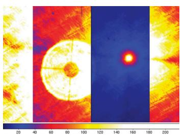
Figure 1: The laser spot imaged with SOI. The SOAR telescope was focused to 7 km to have an in-focus laser spot. Next to the laser spot is an out-of-focus image of a bright star.
