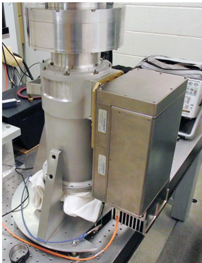
Figure 2: A fully assembled TORRENT controller mounted on a CCD Dewar in the NOAO Tucson detector laboratory. The Dewar contains the science grade e2v CCD for KOSMOS. The detector performance is currently being optimized in preparation for delivery of KOSMOS to KPNO in the very near future. The shiny cylinder bolted to the top of the Dewar contains the Fe-55 radiation source used in the optimization process. (Image credit: Ron George/NOAO/AURA/NSF.)
