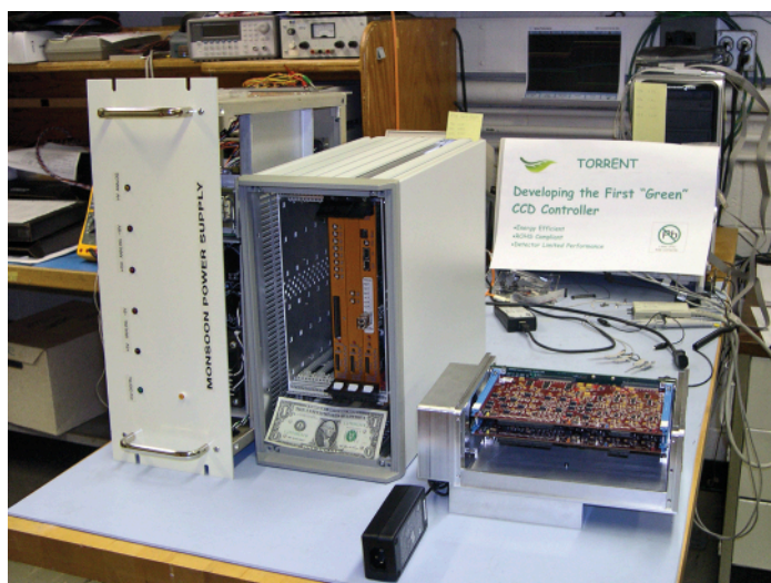
Figure 1: Size comparison between a TORRENT controller (right) with its power supply (small black "brick" in foreground) and a MONSOON unit (middle) with its rack-mountable power supply (left). Both controllers pictured support eight video input channels and achieve the same readout speeds, readout noise, and other detector performance characteristics. (Image credit: Mark Hunten/NOAO/AURA/NSF.)
