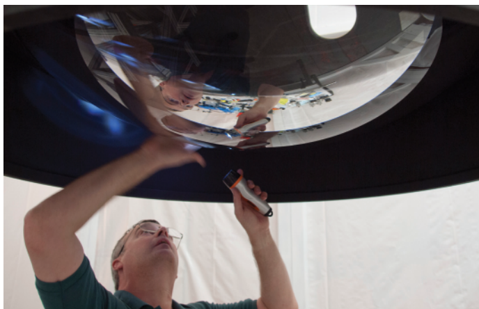
Figure 2: David Brookes of UCL examines and cleans the front surface of the C1 lens. (Image credit: Tim Abbott/NOAO/AURA/NSF.)
