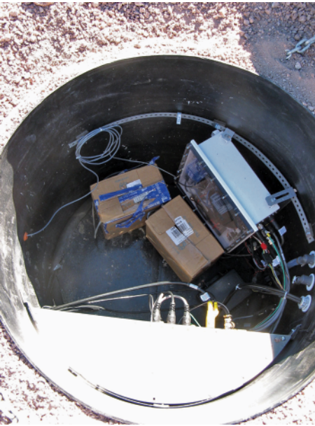
Figure 4: The equipment of the Global Seismic Network in the IRIS seismic measuring station on Cerro Tololo. For more information see: www.iris.edu/hq/programs/gsn/instrumentation . (Image credit: Nicole van der Blik/NOAO/AURA/NSF.)
