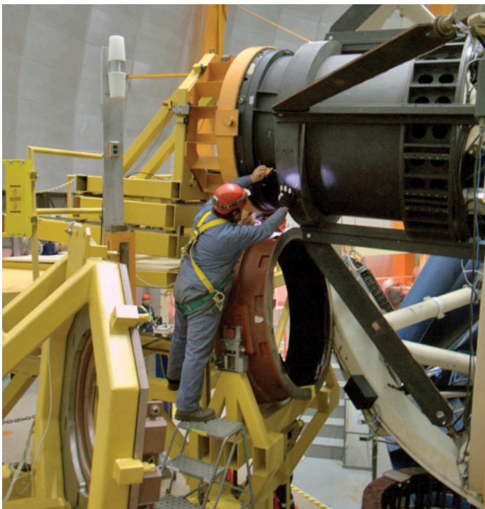
Victor Pinto tightens the bolts attaching the f/8 cell to the prime focus cage. The “red” counterweight is in front of him.
