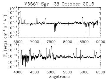
Figure 3: The full spliced spectrum (75 spectral orders) of V5667 Cen (V=13.3) taken with CHIRON on the night of 28 October 2015. The flux axis is logarithmic. The exposure time is 30 minutes. No sky has been subtracted. The data are not smoothed, but the pixel size has been linearized to preserve the resolution at the blue end and hence is very oversampled at the red end.
