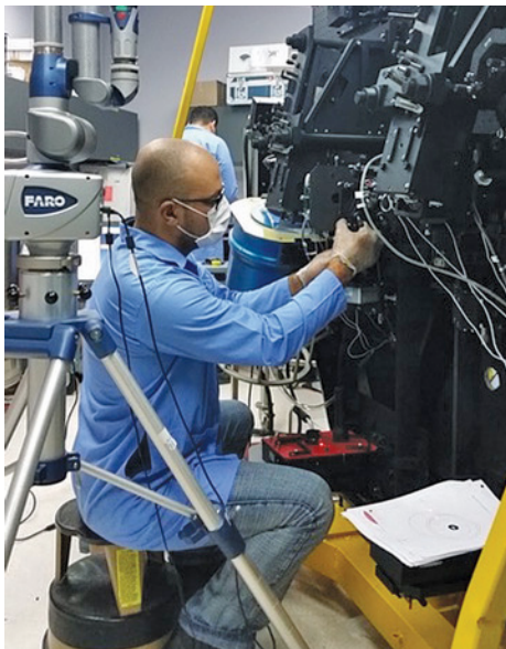
Figure 2. STELES optical alignment. LNA staff working in the SOAR optics lab to realign the instrument after shipment and reassembly. (Image credit: L. Fraga/Laboratório Nacional de Astrofísica.)
