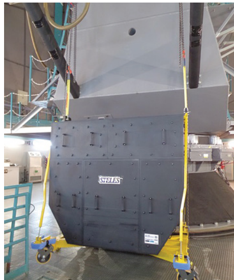
Figure 3. Test lift of the assembled instrument. STELES will mount on the face of the telescope yoke at a point near the top of the photo, just below the optical Nasmyth platform. (Image credit: A. Tokovinin/NOAO/AURA/NSF.)
