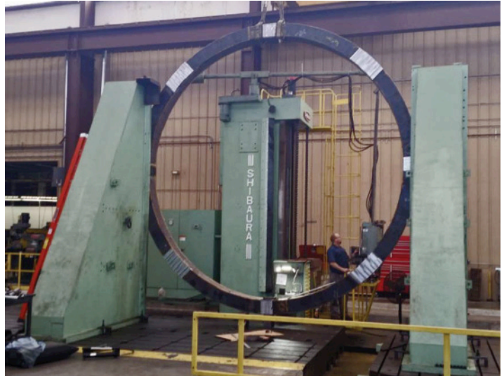
Figure 2. The new top ring for the Mayall telescope, under construction. This will replace the existing, double top ring. (Image credit: DESI Collaboration.)
