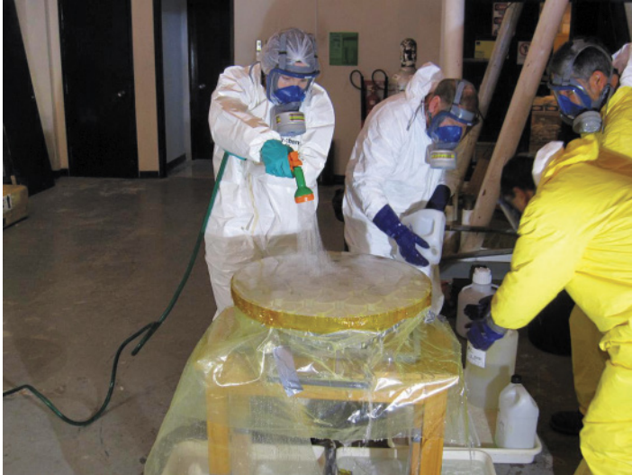
Figure 1. Rinsing the secondary mirror (M2) prior to installing it in the coating chamber. (NOAO/AURA/NSF)
