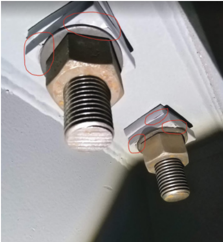
Figure 2. Inside the SOAR telescope yoke showing displacement of bolts, which lifted paint where they shifted. (J. Piracés/NOAO/AURA/NSF)
