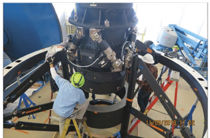
Figure 2. The corrector with hexapod being installed in the top end cage. (NOAO/AURA/NSF)
