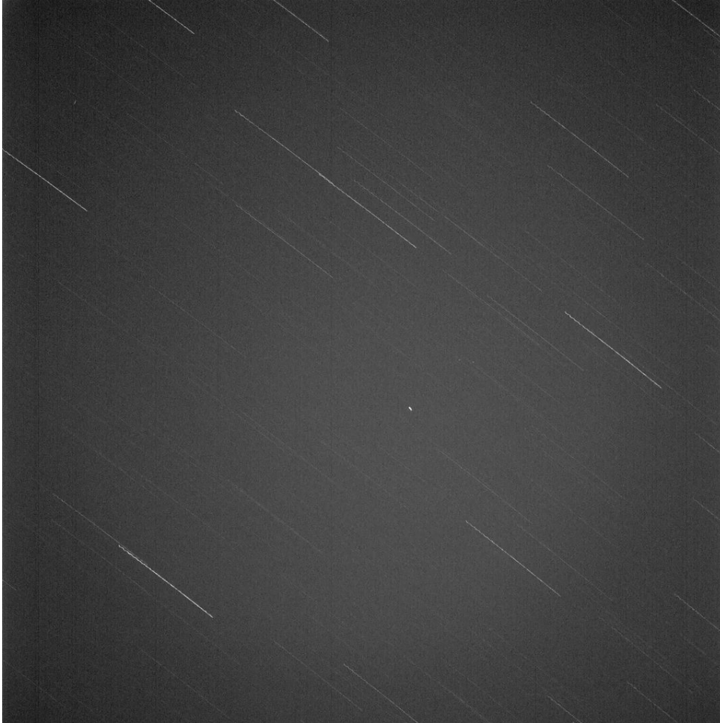
Figure A.2. Starlink-1130 being tracked by the Pomenis Observatory on 16 May 2020. The background stars are severely trailed and often overlap making relative photometry very difficult to do accurately.
