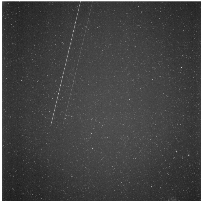
Figure A.5. Starlink-1021 (top) and Starlink-1049 (bottom) as imaged by the Pomenis Observatory on 20 Feb 2020. Although these two satellites are at the same range and flying side-by-side, 1049 is significantly darker. This is likely due to differences in orientation at the time of observation and demonstrates how large an impact orientation has on the apparent brightness.
